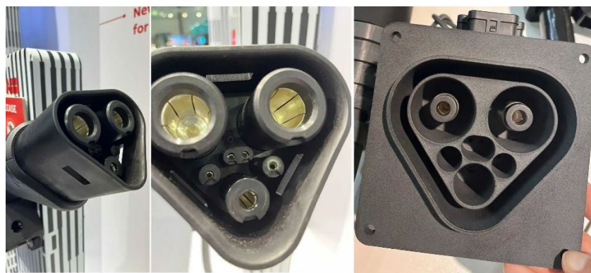
Figure 19. The Megawatt Charging System (MCS) Connector
