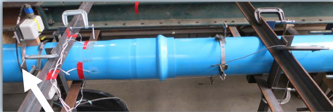
Spigot Compressed into Bell
