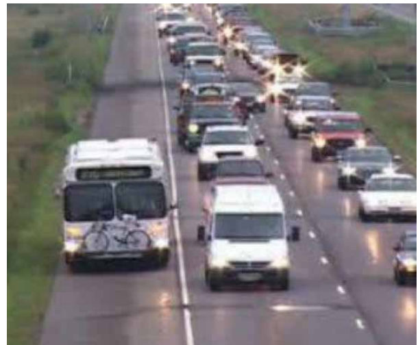
Figure 1-6: Bus-on-Shoulder operation in Minnesota
